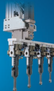
Connecting rod handling achieved with a customized SCHUNK gripping system.
