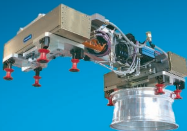
Rim handling with a customized SCHUNK long-stroke gripper.
