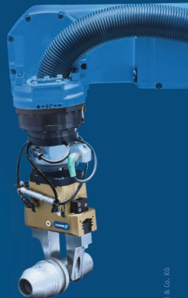
End-of-arm solution. Cast parts handling with SCHUNK standard components
